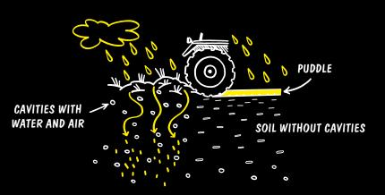
COMPACTED SOIL HAS NO CAVITIES; IT HAS NO SPACES FOR AIR OR WATER.
